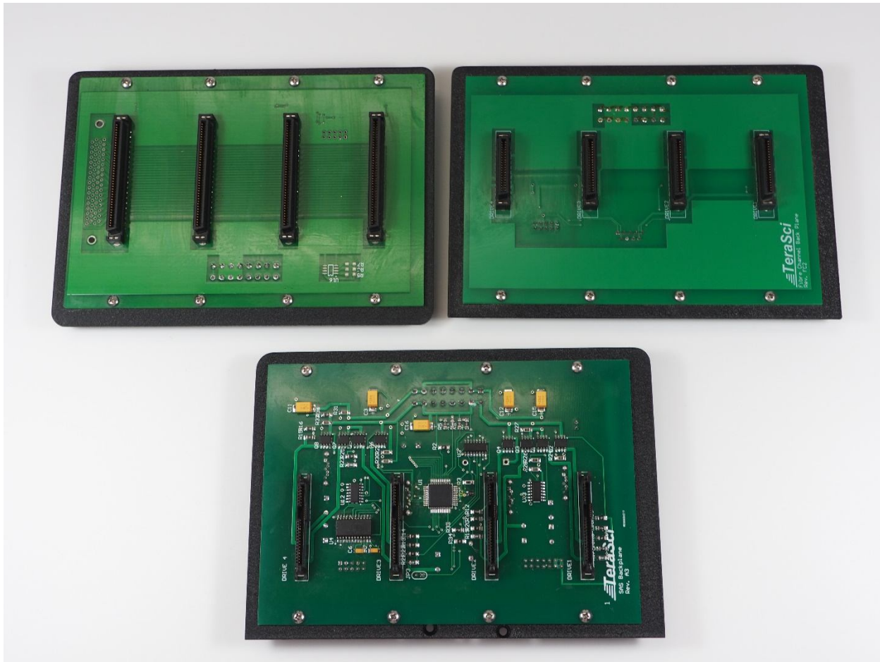
This is a picture of the three backplanes. Top left is the SCSI, top right the FC and at the bottom the SAS backplane.
